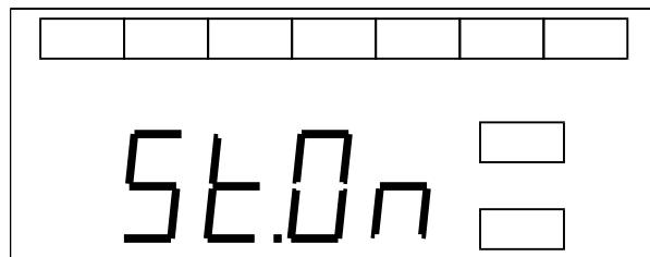
The left part of the display shows which option is selected. To move on to the next option, turn the Adjust knob clockwise.
